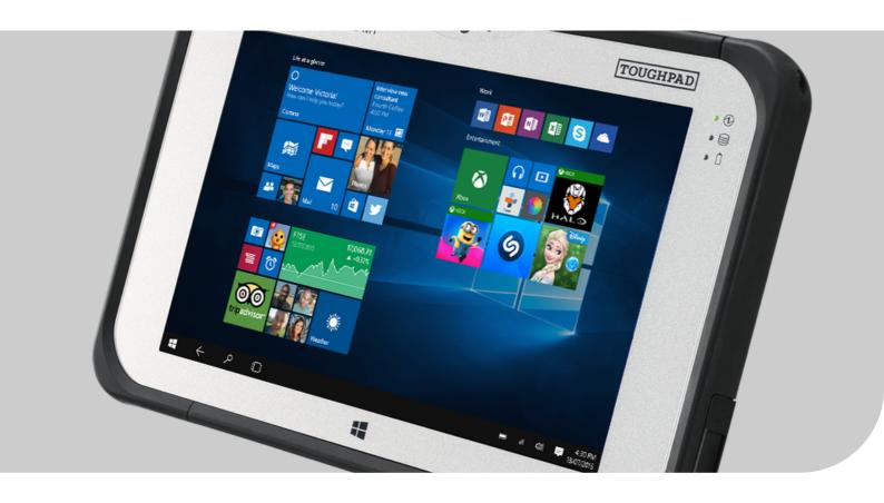
Pocket Size, fanless, fully rugged Windows 10 Pro Tablet with 7" Outdoor Display
