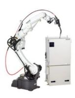
The TAWERS-WG4 Arc Welding System is suitable for CO2, MAG, MIG and Stainless Steel welding applications.
