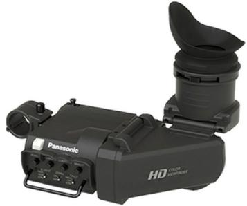
The AJ-CVF25GJ electronic viewfinder is designed to mount on a shoulder ENG camera recorder or studio camera.
