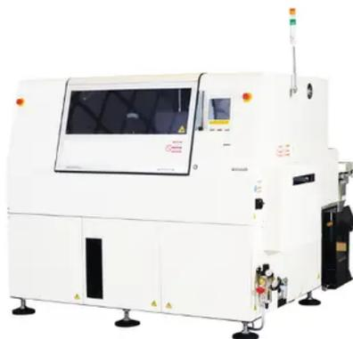
**High speed radial lead component insertion machine for high efficiency and high quality production with high-speed insertion of 0.14s/ component**
