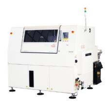
The RL132 high-speed radial THT-insertion machine, with a cycle time of 0.14 s/component, offers outstanding technology in an efficient footprint.
