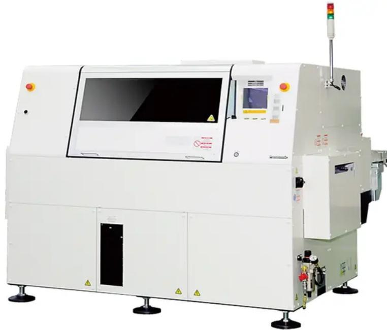
**High density radial lead component insertion machine for high quality and high production with our company's unique insertion method**
