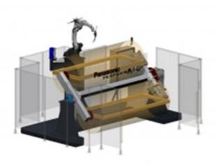
The Panasonic arc welding robot cell PERFORMARC FW-3PD (with 3 external axes PanaDice) is of a modular concept, developed using standard reliable Panasonic components.
