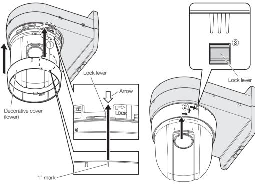
3 Ensure that the lock lever is securely inserted into the hole of the decorative cover (lower).
