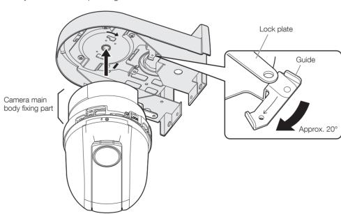
\* Be sure to mount it with holding the camera main body fixing part.
