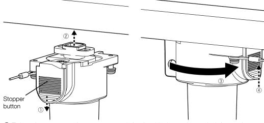
2 Tighten the two screws that were temporarily fixed and fix this product to the lighting rail.
