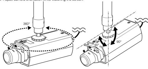
3 Turn the hexagonal hole with a hexagonal wrench to tighten of the movable part of this product. 3 mm {1/8 inches} hexagon wrench (locally procured)
