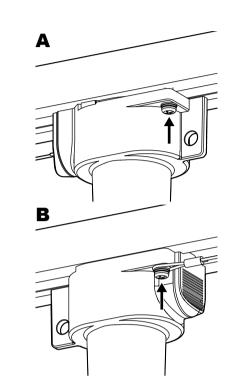
After fixing this product to the lighting rail, be sure to check that the safety wire from the camera is not in contact with the inside of the rail (energized part).
