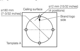
Step 2 Install two anchor bolts (M10: locally procured) into the ceiling.
