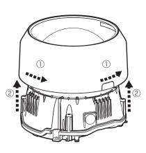
Connect the cables and mount the camera on the attachment plate. Refer to the installation guide or the installation procedure leaflet of the camera for connection of cables and for how to fix the camera.
