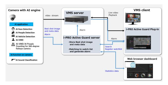
Al application or Al function on cameras transmit video stream to VMS server and transmit Best shot images and meta data to i-PRO Active Guard server.
