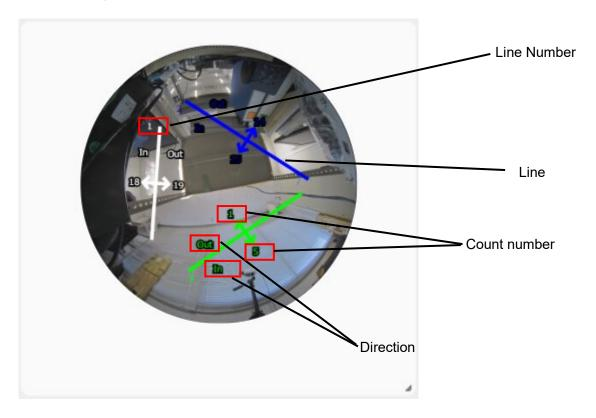
**Line:** Displays the position of the cross line set on the camera.
