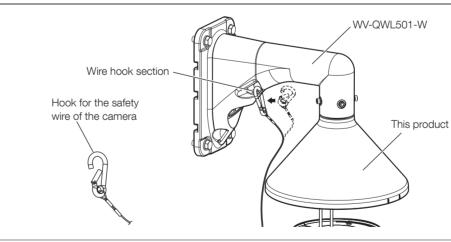
When connecting the safety wire to WV-QCL501-W, follow the procedure below to attach the safety wire to WV-QCL501-W.
