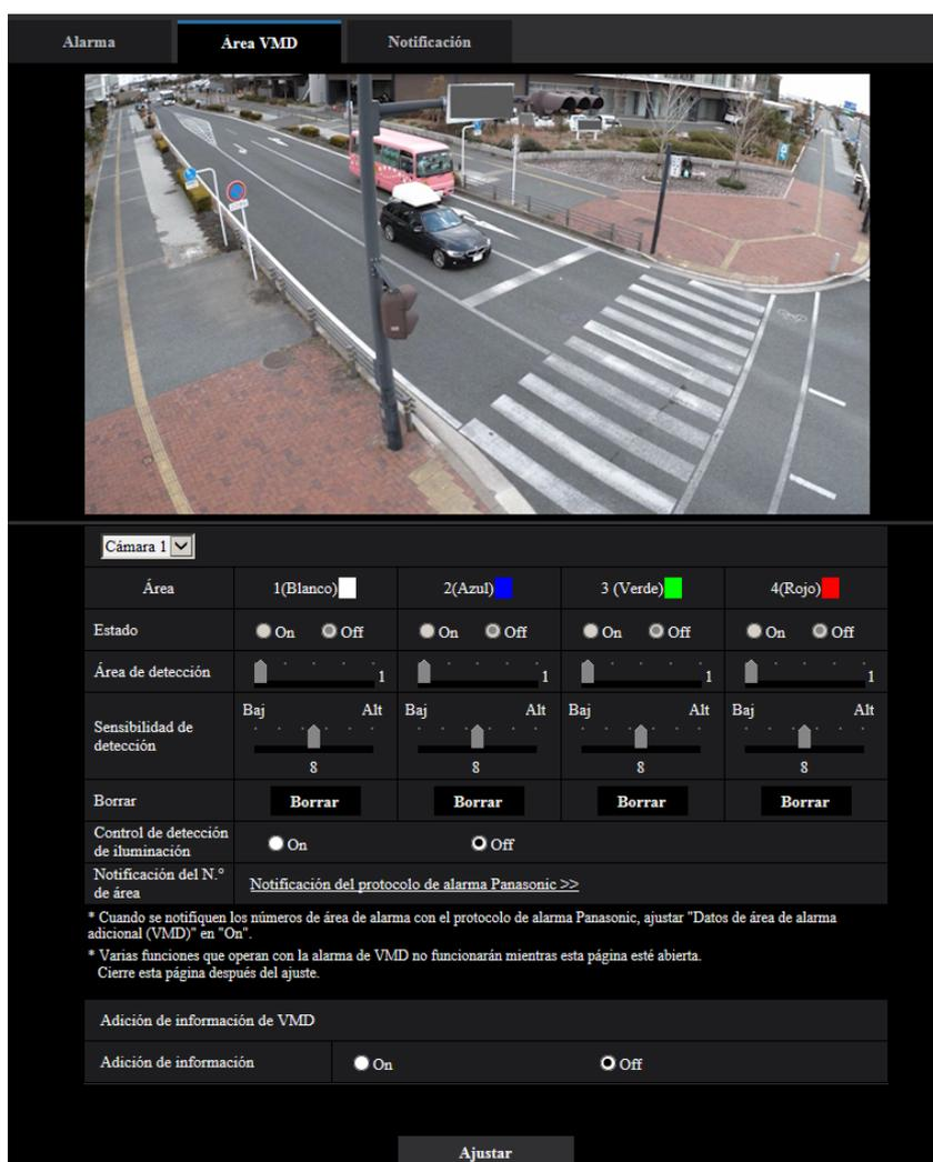
The screenshot displays the VMD configuration interface. At the top, there are three tabs: "Alarma", "Área VMD" (selected), and "Notificación". Below the tabs is a live camera feed showing a street scene with a car and a bus. The interface is divided into several sections:
