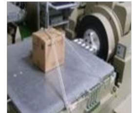
■ Box Shaking Test
