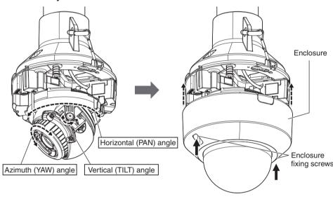
Recommended tightening torque : 0.59 N·m {0.44 lbf·ft}
