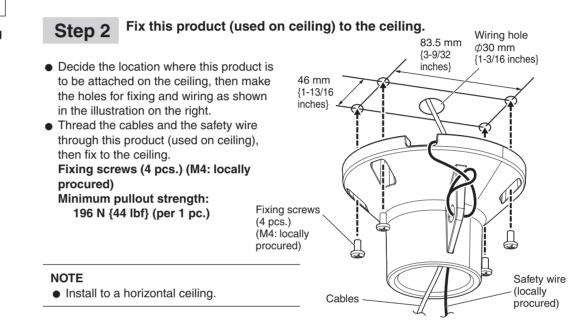
■ The following explanation describes an example of attaching an indoor dome type WV-S2131L model
