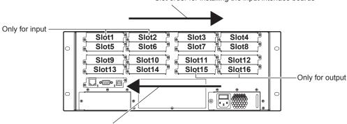
Slot order for installing the output interface board
