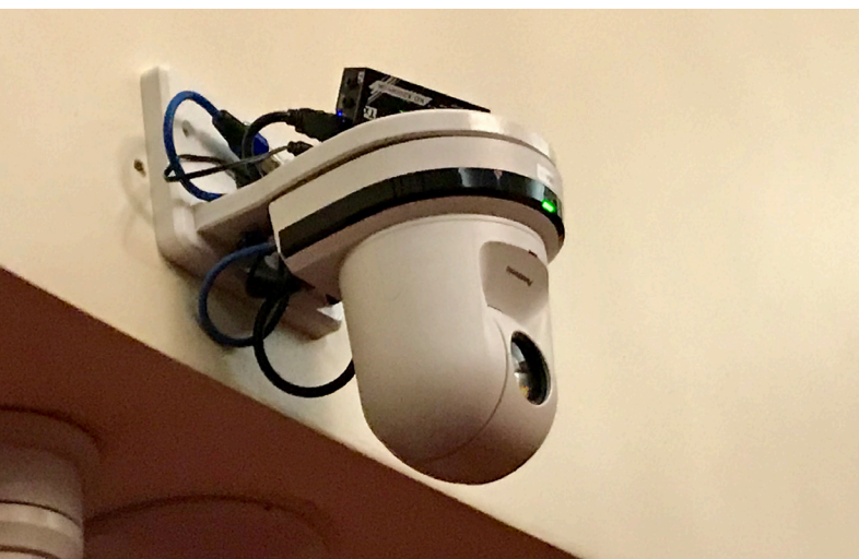
The church chose the AW-HN38 PTZ camera based on built-in NDI support.
