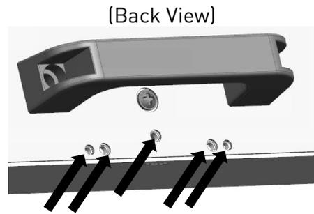
2. Tighten two screws to plate.
