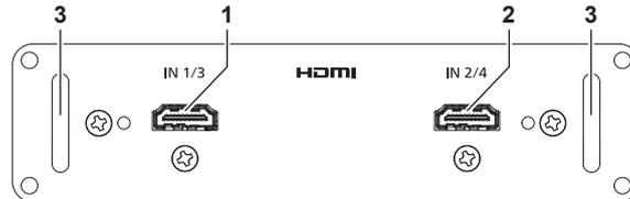
1 <HDMI IN 1> terminal (when installed in <SLOT 1>), <HDMI IN 3> terminal (when installed in <SLOT 2>)
