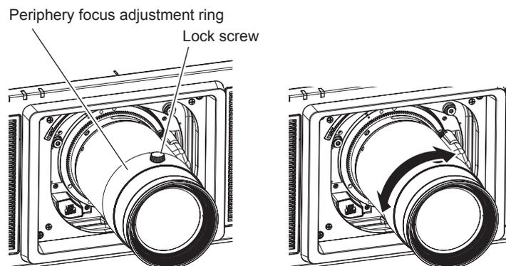
**3) Check the focus at the center of the image again and make fine adjustments.**
