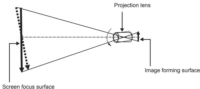
**How to adjust the focus balance (adjustment by tilting the lens mounter)**
