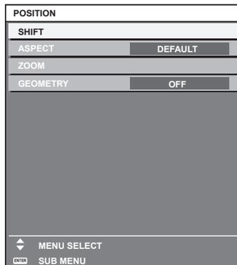
4) Press ▲▼ to select a sub-menu, and press ◀▶ or the <ENTER> button to change or adjust settings.
