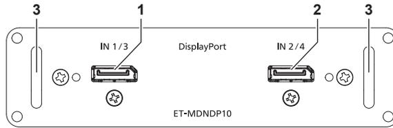
1 <DisplayPort IN 1> terminal (when installed in <SLOT 1>),
