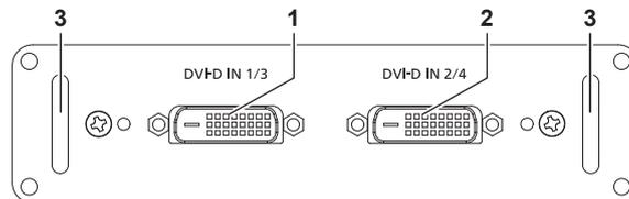
1 <DVI-D IN 1> terminal (when installed in <SLOT 1>), <DVI-D IN 3> terminal (when installed in <SLOT 2>)
