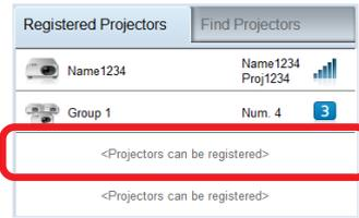
When [<Projectors can be registered>] on the <Registered Projectors> screen is clicked, the <Register Projectors> screen is displayed.
