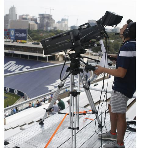
*"In making our camera choice, the initial top criterion was uncompressed long-distance transmission over SMPTE fiber, an ESPN3 design spec. But once we made the decision to invest in 4K now, the UC3000 won out not only on the basis of that capability, but also its attractive price point and 4K/HD image production."*
