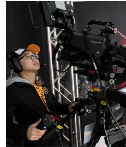
RIT has recently upgraded its production studio with the addition of Panasonic AK-UC3000 4K/HD studio camera systems and AW-HE130 pan/tilt/zoom cameras. The studio features six AK-UC3000 4K/HD camera systems as main cameras, ten AW-HE130 FHD pan/tilt/zoom cameras and several LCD broadcast monitors for production, engineering and camera shading. All operate under in-arena IP control, complementing these cameras' capabilities.
