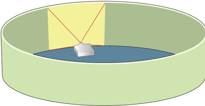
Images are corrected to fit a screen whose shape is elliptical when viewed from above.
