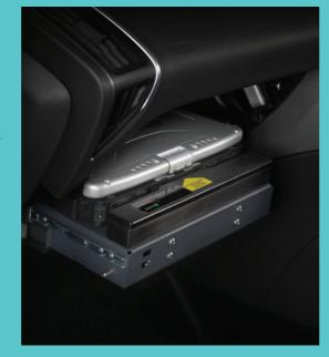
PANASONIC DOCKS CAN BE DASHBOARD-MOUNTED, STORED IN THE REAR OF THE VEHICLE OR HIDDEN OUT OF SIGHT, FOR EXAMPLE IN THE GLOVE BOX.
