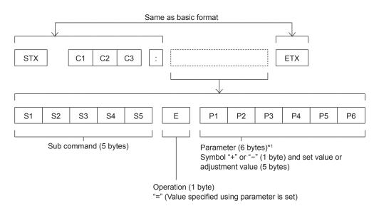
\*1 When transmitting a command which does not need a parameter, the operation (E) and parameter are not necessary.
