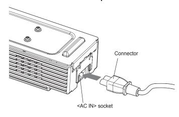
Check the shapes of the <AC IN> socket of the projector and the connector of the power cord and then orient the connector correctly and insert it firmly.
