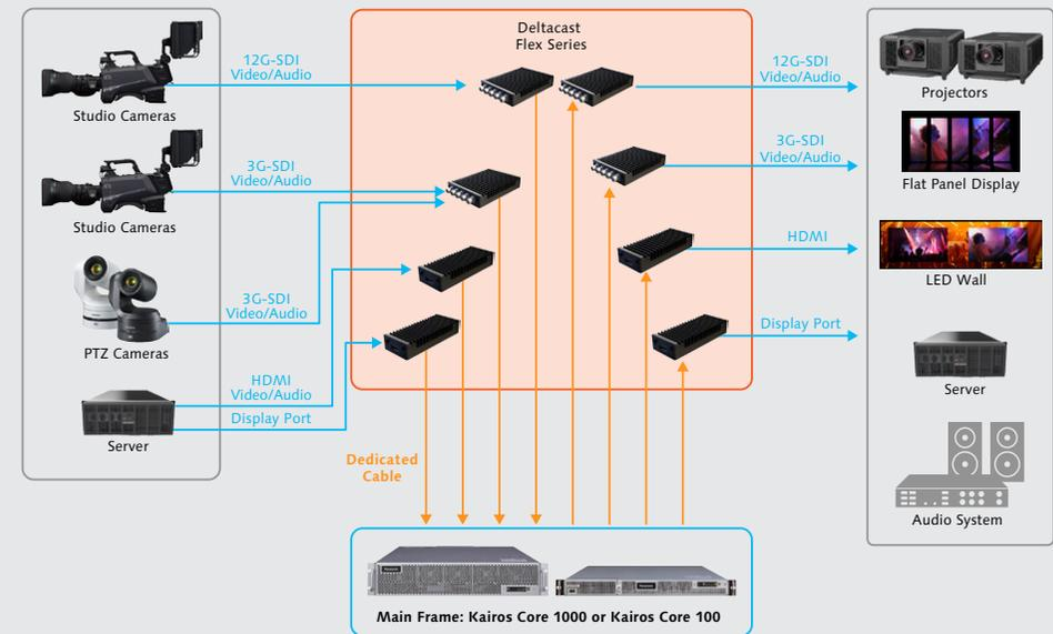
\*Deltacast FLEX modules are required for baseband input/output.
