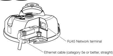
Connect an Ethernet cable (category 5e or better, straight) to the RJ45 Network cable or RJ45 Network terminal.
