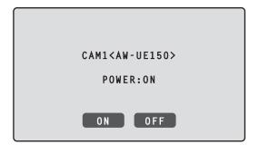
Turning on the power of the cameras simultaneously with the turning on of the unit's power
