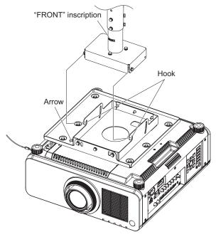
2) Insert the temporarily fastened captive washer hex head bolts on either side into the hook section of the angle adjusting bracket.
