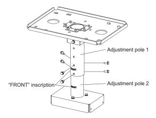
Insert the adjustment pole 1 into the adjustment pole 2, align the holes, and secure them with the supplied six captive washer hex head bolts (M6 × 16).
