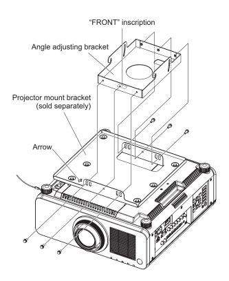
Secure the angle adjusting bracket to the projector mount bracket using the six supplied captive washer screws (M6 x 16) as illustrated on the left.
