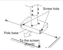
1) Screw the supplied two captive washer hex head bolts (M6 × 16) half way into two opposite side bolt holes in the pole base, on the forward side nearest the screen.
