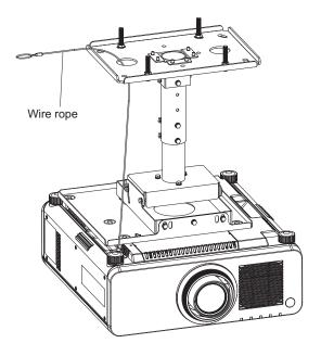
4) Pass the wire rope through the hole of the attachment plate as illustrated on the left.
