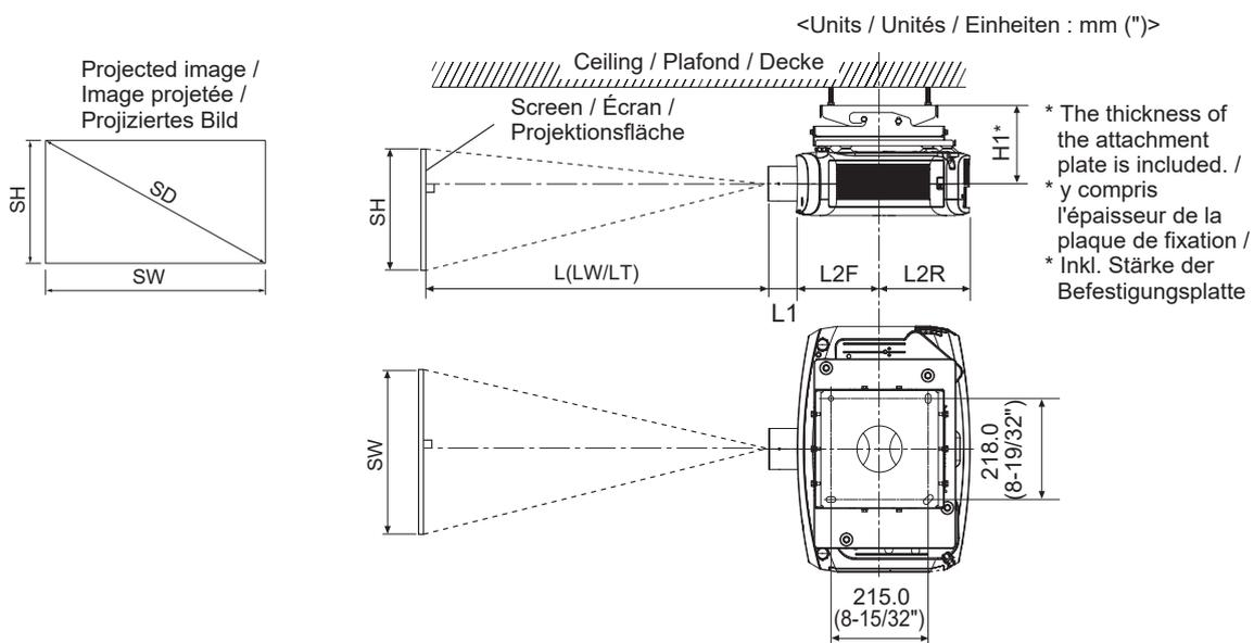
(when using the ceiling mount bracket ET-PKD120H (for high ceilings))
