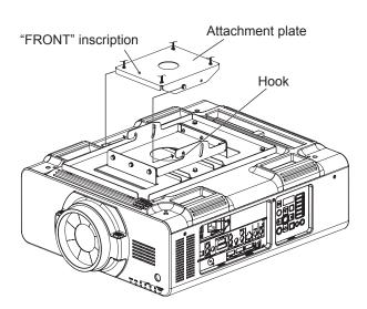
Screw the supplied two captive washer hex head bolts (M8 × 20) half way into two opposite side bolt holes in the attachment plate, on the forward side nearest the screen.
