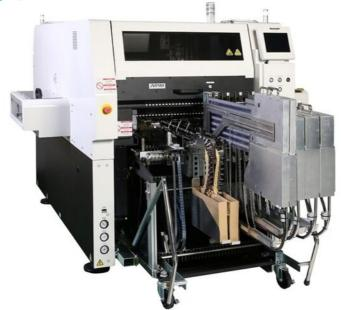
Panasonic's all-rounder pick-and-place machine that handles both SMT and THT components as standard or odd-form components in one placement order.
