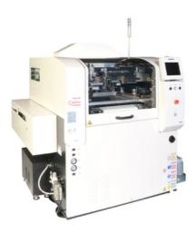
The high-speed printer SPV features an average print cycle time of just 10s for precise SMD-printing, PCB-transfer, recognition and stencil-cleaning.
