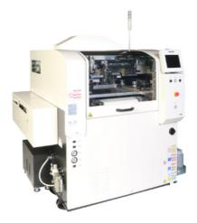
The high-speed printer SPV features an average print cycle time of just 10s for precise SMD-printing, PCB-transfer, recognition and stencil-cleaning.
