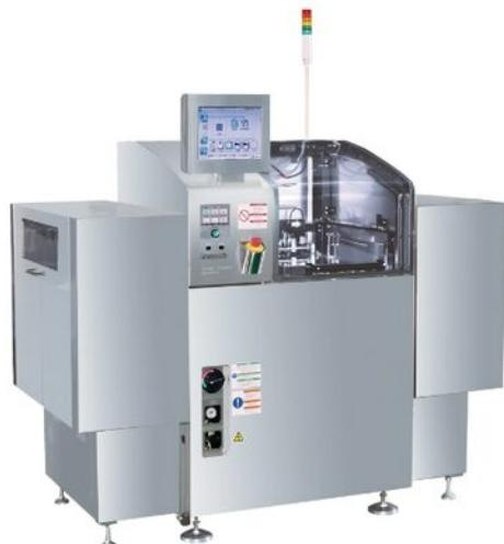
**Plasma cleaning utilizing parallel plate plasma cleaning technology.**
