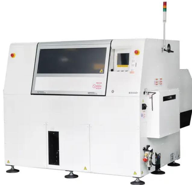
**High speed axial lead component insertion machine for high productivity with High speed insertion of 0.12 s / component , sequential component supply system and vertical automated feeder**
