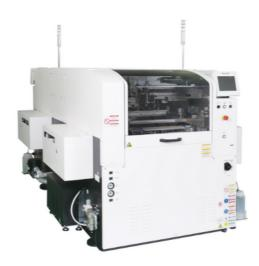
With two lanes, the SPV-DC features high precise SMD-printing, PCB-transfer, recognition and stencil-cleaning for high volumes without changeover time.
