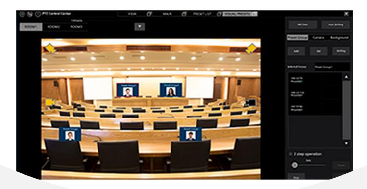
GUI screen that enables the subject of multiple PTZ Cameras to be switched with a single click of an icon
