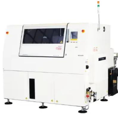
**High speed radial lead component insertion machine for for high efficiency and high quality production with high-speed insertion of 0.14s/ component**
