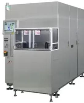
**A dry etching system specializing in the processing of chemical compounds and non-volatile materials**
