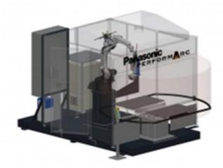
The Panasonic arc welding robot cell PERFORMARC MT (Manual Turntable) is of a modular concept, developed using standard reliable Panasonic components.
