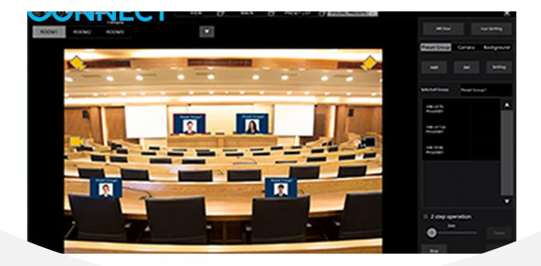
GUI screen that enables the subject of multiple PTZ Cameras to be switched with a single click of an icon
