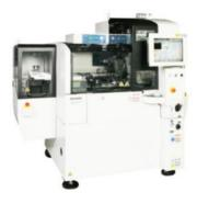
High accuracy, high quality, ultrasonic flip-chip device bonding.
